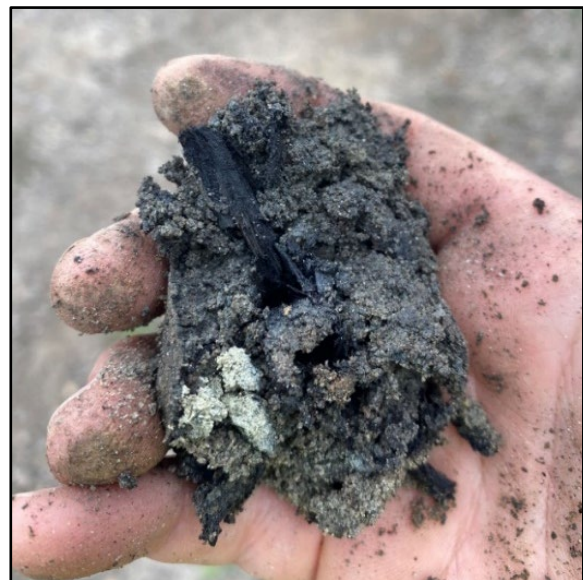
Figure 4-3. Fill in Boring B-2
