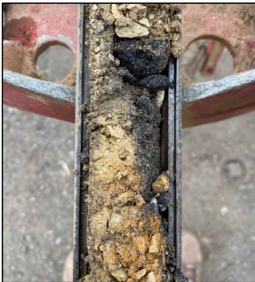
Figure 4-2. Fill in Boring B-1
